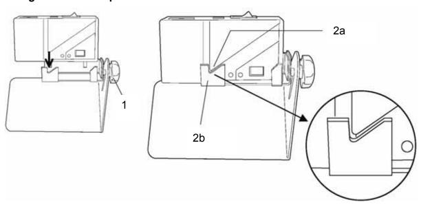
Position knob (1) and tighten it by turning. Insert the ionizer into the V-shaped recess (2a → 2b), ensuring a good fit
