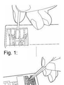
Do not use aggressive cleaning agents (solvents etc.) instead clean with a soft cloth soaked in mild soap suds. Take care that the device is not penetrated by fluids and polish it with a dry soft cloth. Remove loose sample residues / powder carefully with
