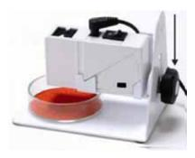
⇒ Discharge of powdery samples. Discharge prevents whirling up, problems with toxic samples.
